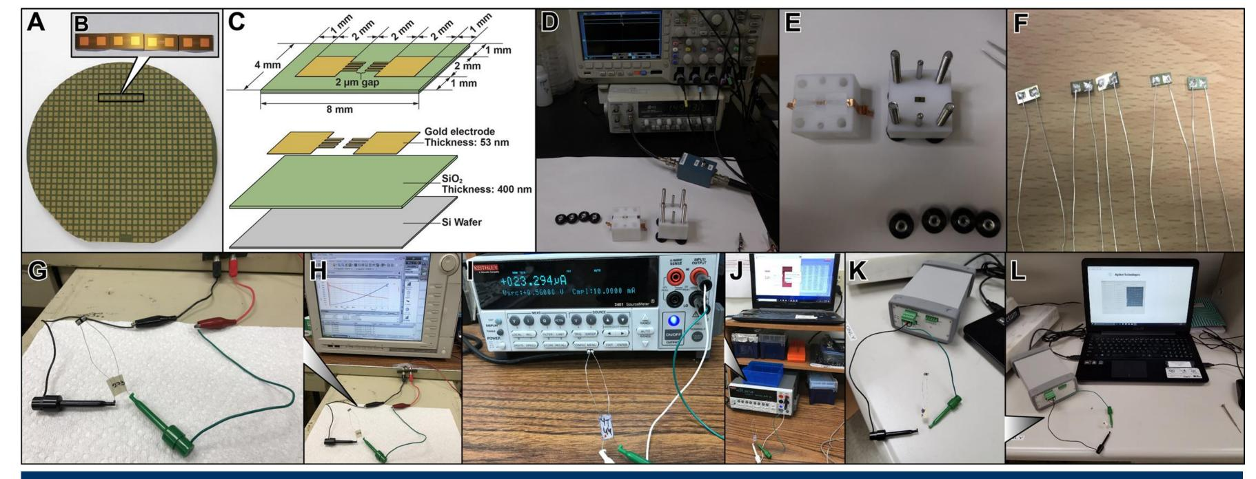
(A) A pre-diced silicon wafer from which the microelectrodes are cut, (B) Magnified to show the microelectronic devices (MEDs), (C) Dimensions of the MED, (D) Nanomaterial deposition station (E) Device in mold for deposition, (F) Soldered devices, (G-H) Agilent Semiconductor Device Analyzer for testing devices, (I-J) Keithley sourcemeter setup for testing devices, and (K-L) Keysight sourcemeter setup for testing devices.
